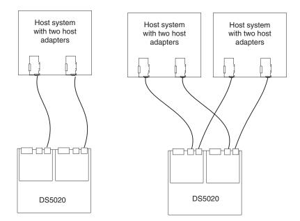
Figure 56. Examples of redundant host direct attached Fibre Channel SAN configurations
